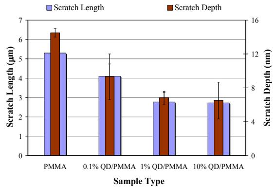
**Figure 3.** Comparisons of the scratch length and depths of the samples.
