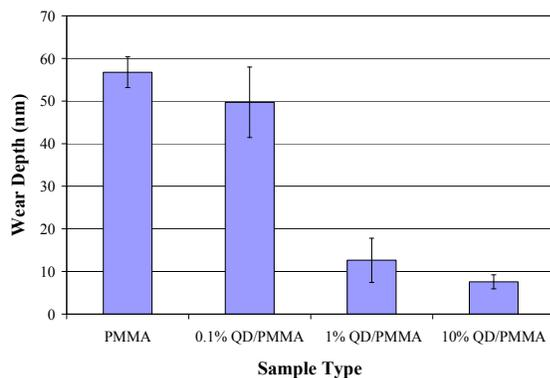
**Figure 2.** Comparisons of the wear depths of the samples.
