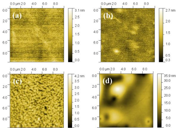
**Figure 1.** SPM surface topography of the samples. (a) PMMA, (b) 0.1%QDs, (c) 1%QDs, and (d) 10% QDs.
