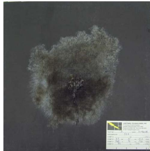
Fig. 1 Surface damage of the panel CE-NCNS-1 after lightning strike test.
