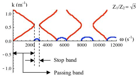
Fig. 1 Frequency band-gap of 1D rod structure
