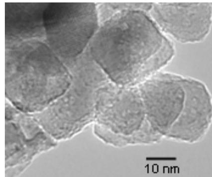
Figure 1. TEM image of 1-2 nm thick nickel coating of a TiO<sub>2</sub> anatase porous electrode..
